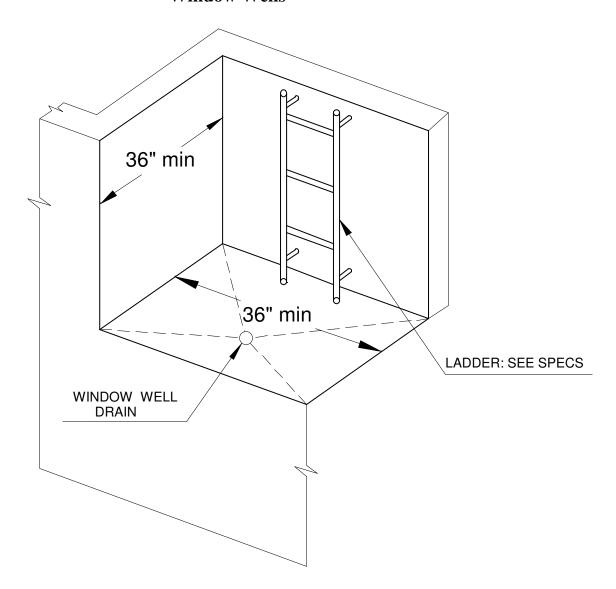
**R310.2** Window wells. Window wells required for emergency escape and rescue shall have horizontal dimensions that allow the door or window of the emergency escape and rescue opening to be fully opened. The horizontal dimensions of the window well shall provide a **minimum net clear area of 9** square feet with a minimum horizontal projection and width of 36 inches.
