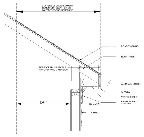
Ice/Water Shield to Be Used in Lieu of 15# Felt Paper at Eaves.
