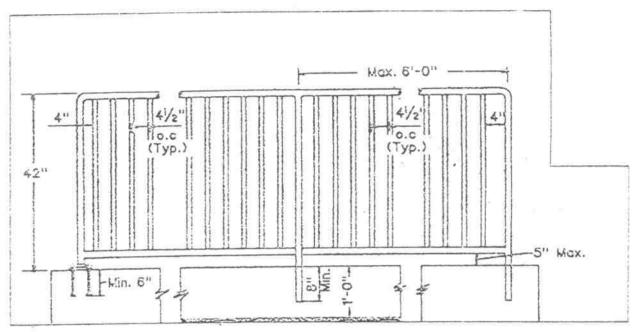
I. HANDRAIL TO BE PRIMED WITH I COAT OF KOPPERS 622 RUST I, PENETRATING PRIMER, OR APPROVED EQUAL, THEN PAINTED WITH 2 COATS OF DURON NEW RETHANE MODIFIED BLACK (OR APPROVED EQUAL). PAINT TO BE APPLIED AT MIN. 1.5 MIL. PER COAT. COLOR TO BE PICKED BY ARCHITECT.
