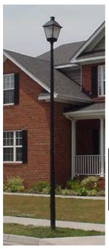
Smooth round tapered composite poles constructed of heavy duty fiberglass reinforced pigmented polyester resin for single pole top luminaires. Poles are directly embedded for use with underground supplied conductors only.
