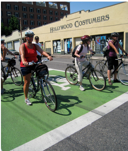
Bike boxes, above left, provide a dedicated space for bicyclists ahead of motor vehicle traffic at signalized intersections. Bicycle crossing markings, above right, provide clear direction for bicycle travel through an intersection.
