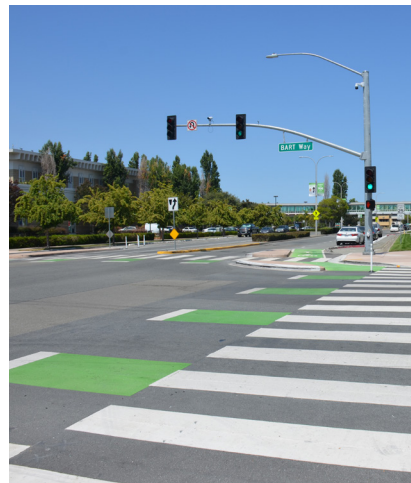
Bike boxes, above left, provide a dedicated space for bicyclists ahead of motor vehicle traffic at signalized intersections. Bicycle crossing markings, above right, provide clear direction for bicycle travel through an intersection.
