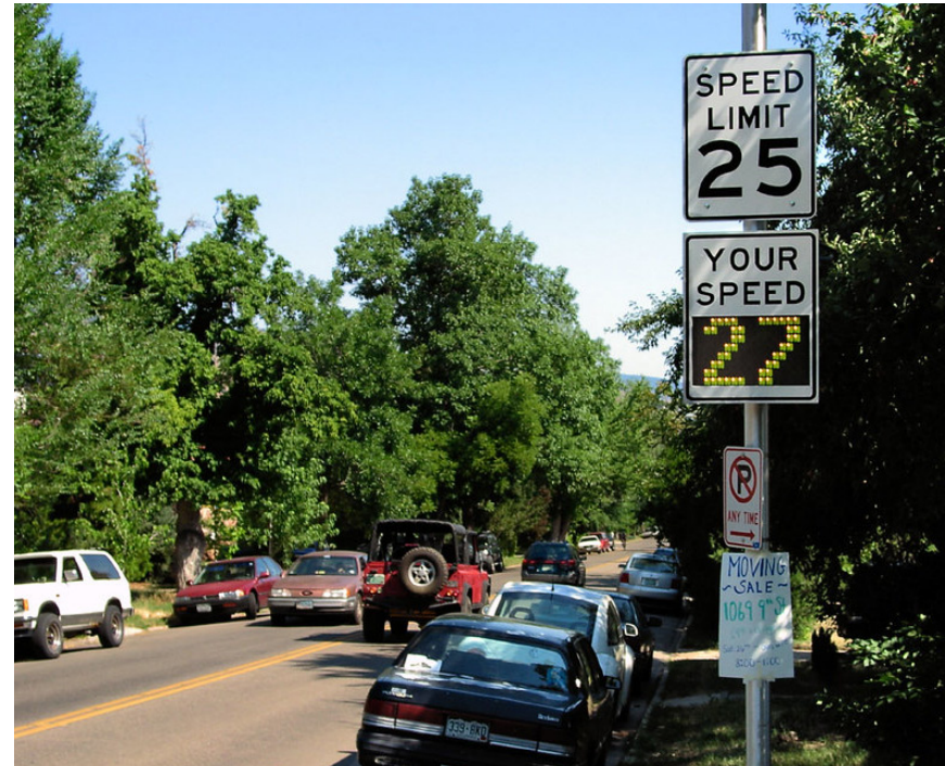
Permanently mounted speed feedback signs can be used to heighten awareness of speed limits.
