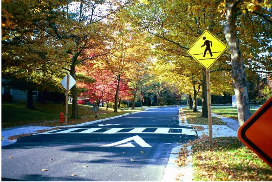
Figure 20. Example of a Raised Crosswalk
