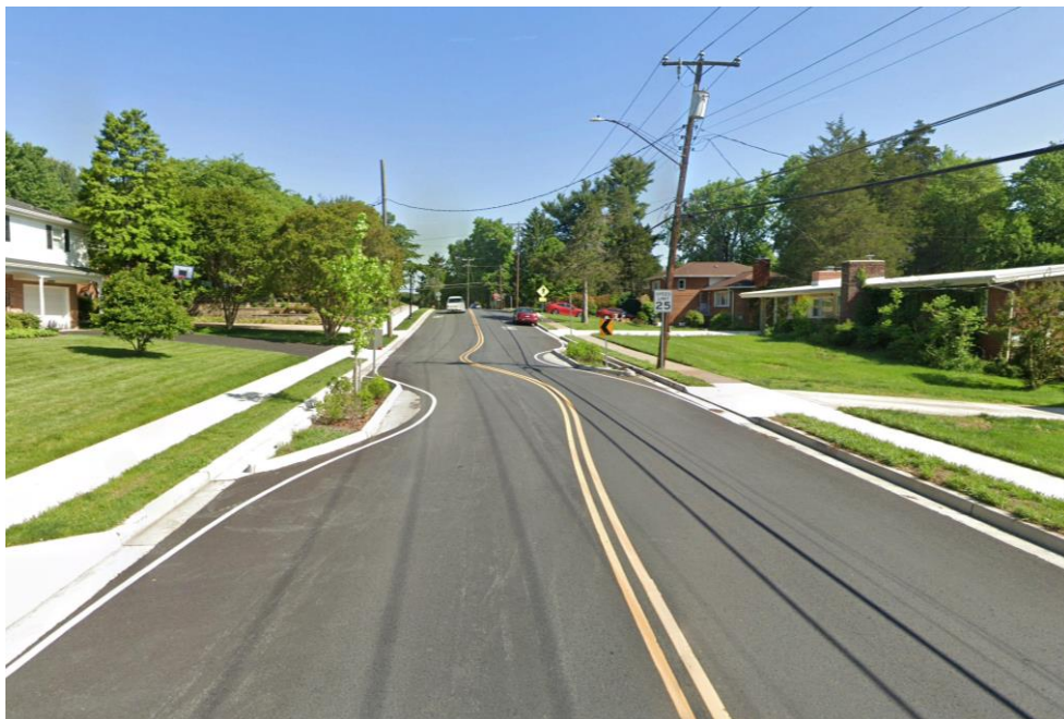
Figure 17. Example of a Chicane
