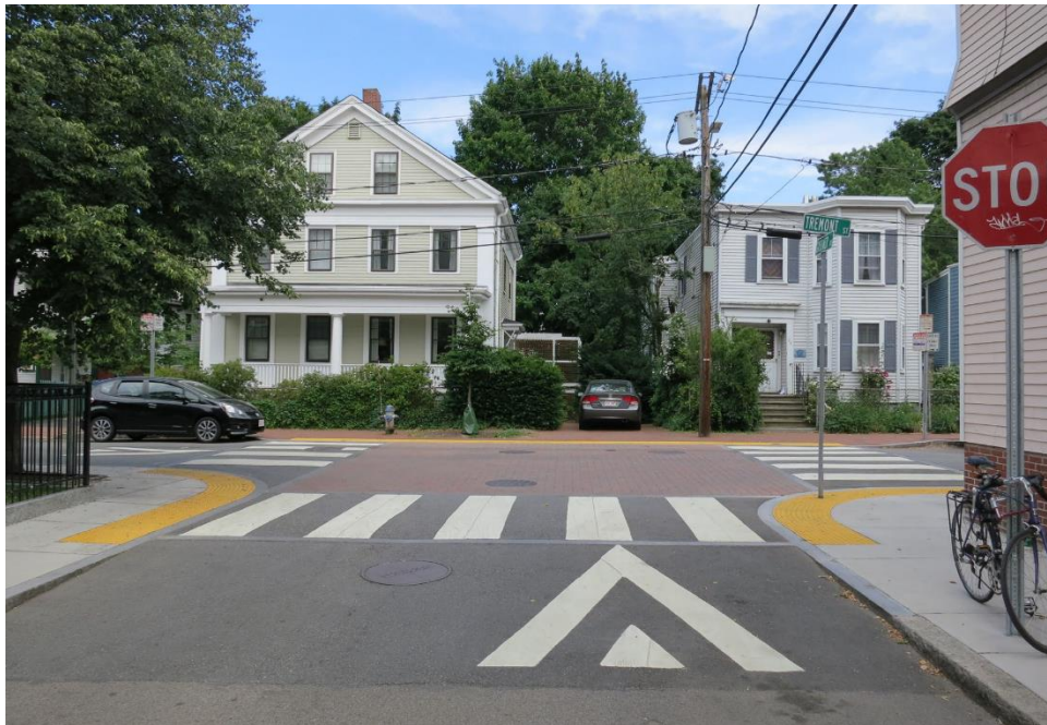
Figure 19. Example of a Raised Intersection
