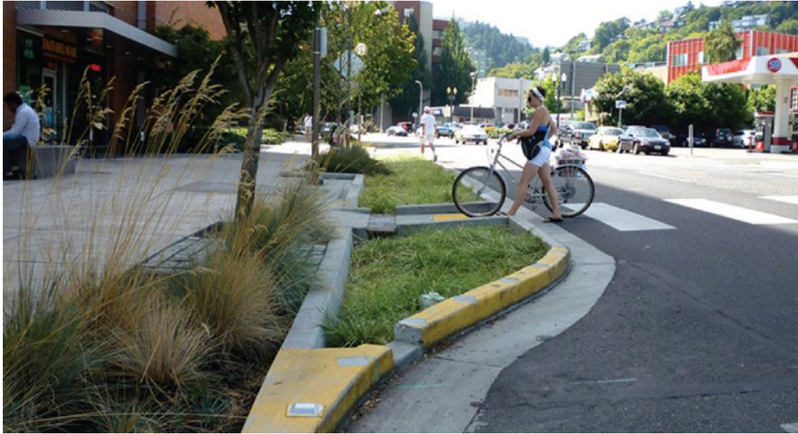
Figure 16. Example of a Curb Extension (Source: NACTO)
