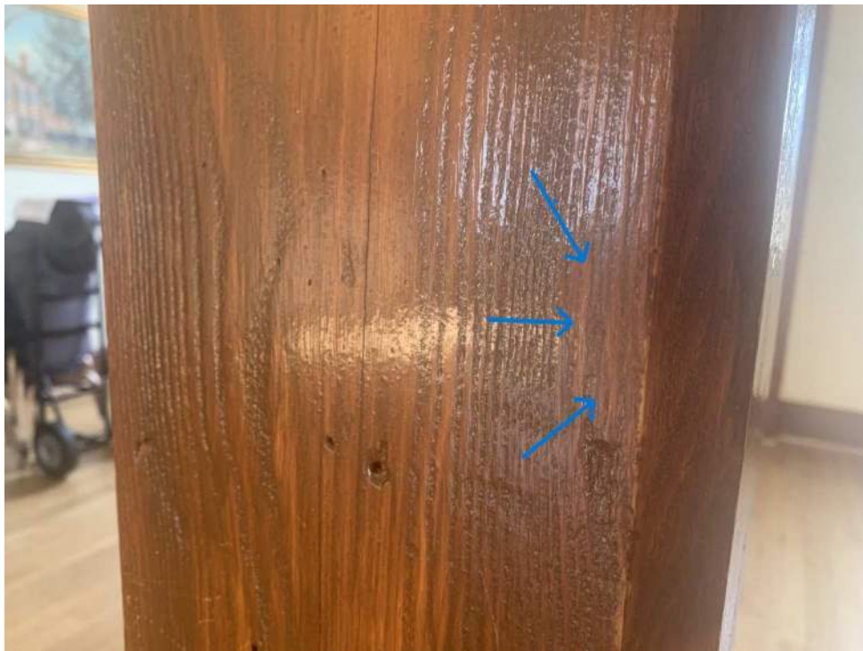
Figure 12: Solvent test results on first-floor Assembly Room (104) column indicating lacquer finish. The test area appears dull where the acetone was applied to the surface.
