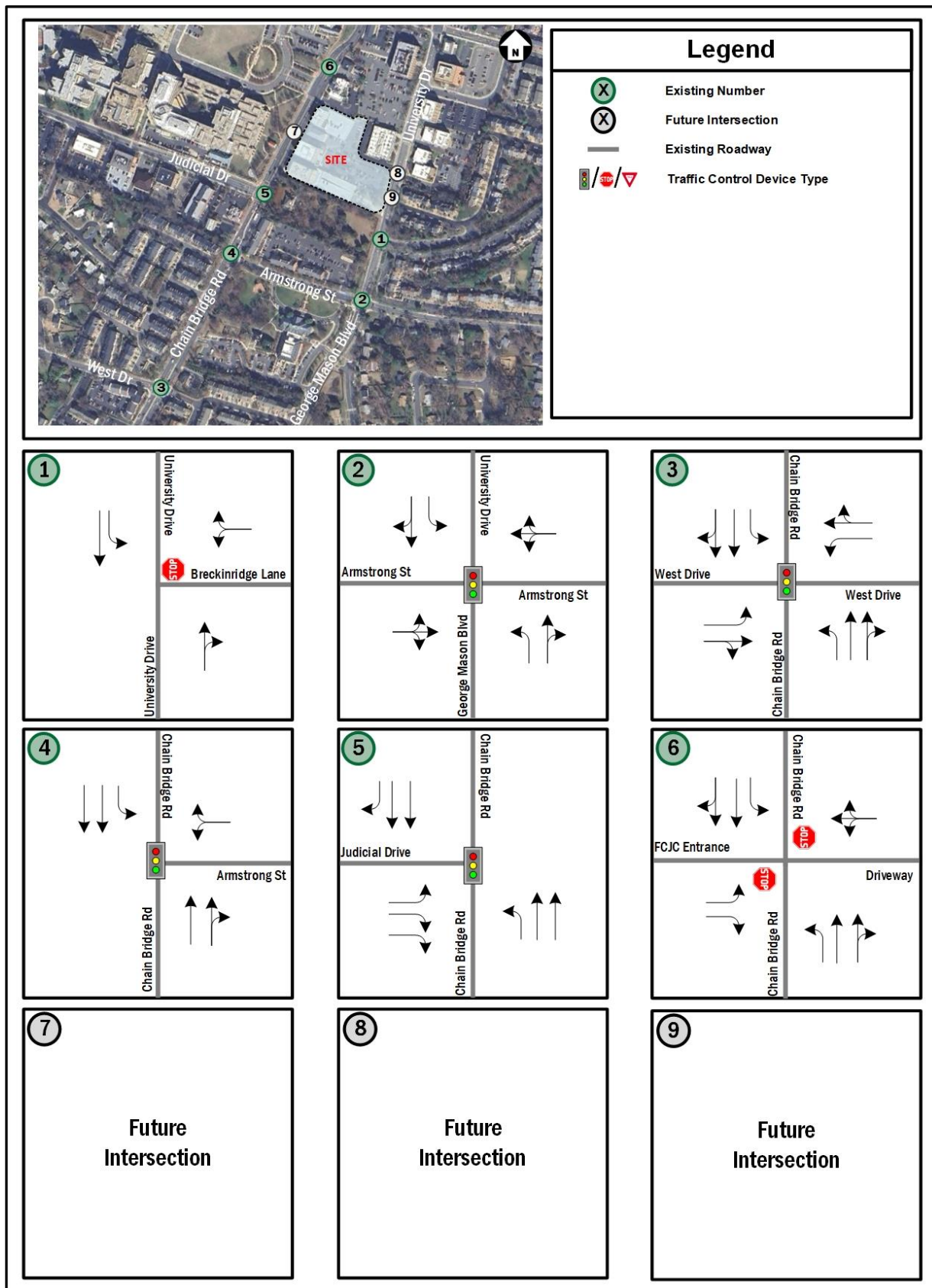
Figure 16: Existing (2024) – Lane Configuration
