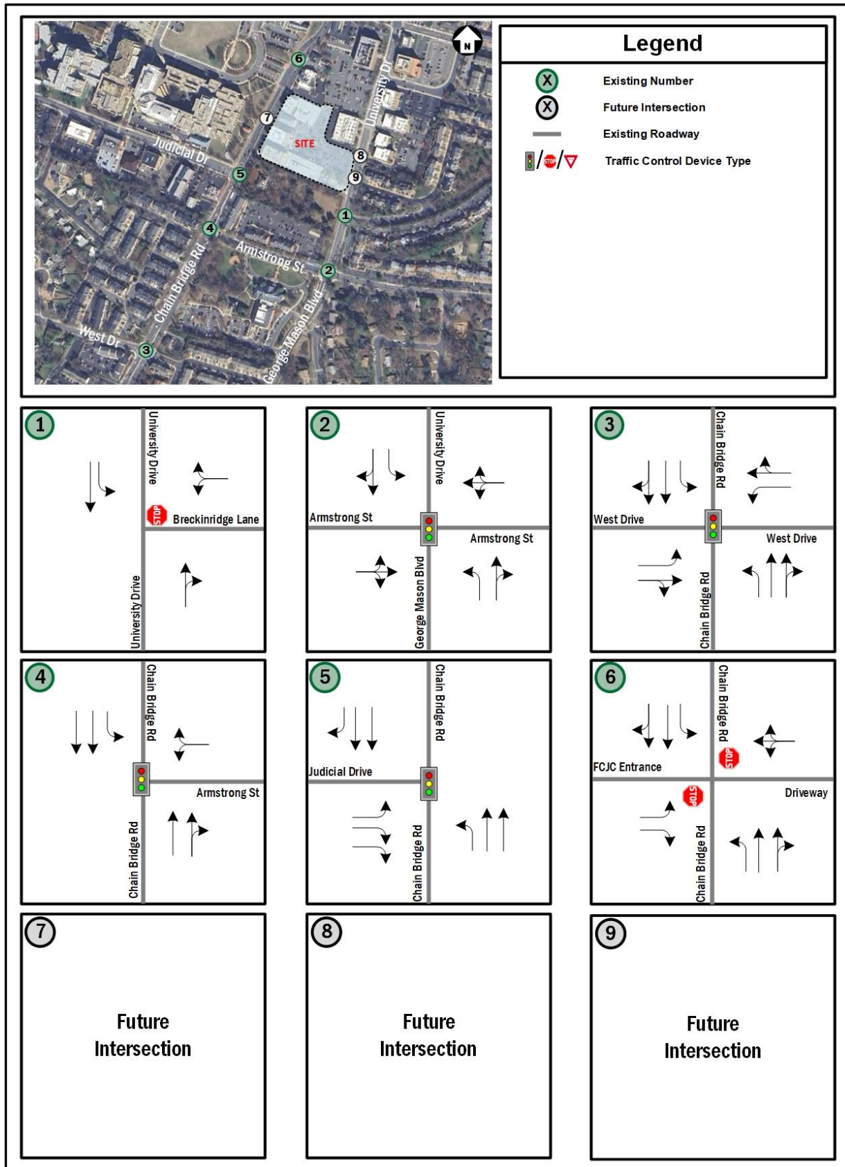
Figure 13: Existing (2024) – Lane Configuration
